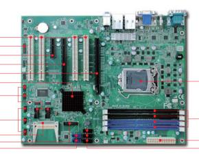
RUBY-D714VG2AR is based on Intel Q77 chipset and desktop processor sku like Core i5 and i7. Build with flexible PCI express expansion and bifurcation feature, it can support two IO interface cards and can also suitable for Medical, Industrial automation, and digital signage applications.
