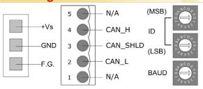
ID: Node ID Baud: Device Baud Rate
