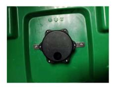
Fix on top of the cover of waste bin, with sensor facing down.
