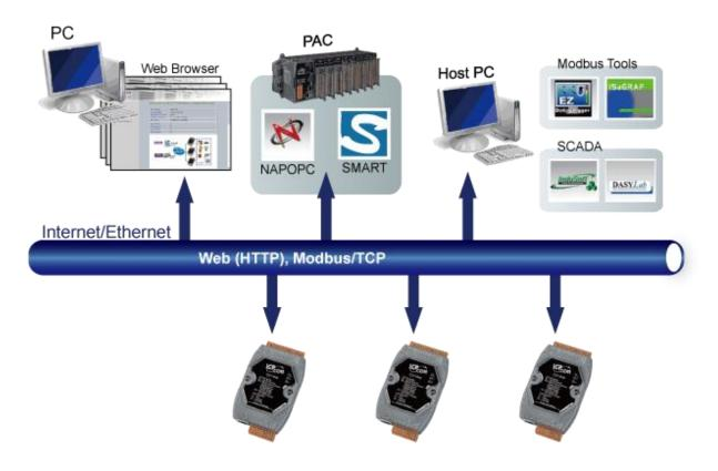
Besides, with the web HMI function, no more programming or HTML skills are needed; creating dynamic and attractive web pages for I/O monitoring and I/O control would be fun to engineers ever after. The ET-7016/PET-7016 offers easily and safely access for users from anytime and anywhere! In addition, ET-7016/PET-7016 also supports Modbus/TCP protocol that makes perfect integration to SCADA software.
