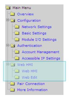
**Web HMI:** Links to the I/O monitor page that allows you to monitor and control the I/O status on ET-7016/PET-7016 module remotely.
