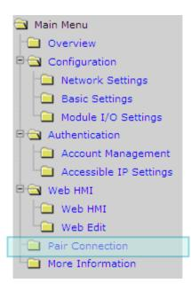
This pair connection function is a particular feature of ET-7016/PET-7016 that can enable a pair of DI-to-DO via Modbus/TCP. With pair connection function enabled, ET-7016/PET-7016 modules can poll the status of remote DI devices using the Modbus/TCP protocol and then continuously write to its DO channels in the background.
