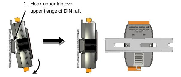
2. Tilt the module toward DIN rail until it snaps securely to DIN
