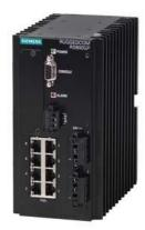
RUGGEDCOM RS900GP is a utility grade, fully managed Ethernet switch providing dual fiber optical or copper Gigabit Ethernet ports and 8 Fast Ethernet copper ports; power over Ethernet, 802.3at 128-bit Encryption; 8 Fast Ethernet Ports (10/100BaseTX) all External 802.3af/802.3at compliant PoE; Up to 2 Fiber Optical Gigabit Ethernet Ports (100/1000BaseX); Up to 2 10/100/1000 BaseTX Multiple fiber connector types (LC, SC,ST, SFP
