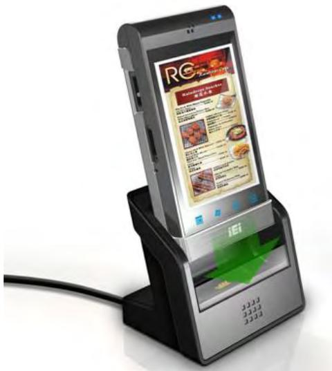
Figure 2-6: Connect the MODAT-200 to the Charging Cradle
