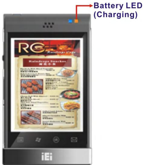
Figure 2-3: Battery LED
