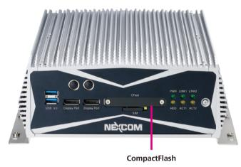
2. Remove the mounting screws and cover of the CompactFlash socket.
