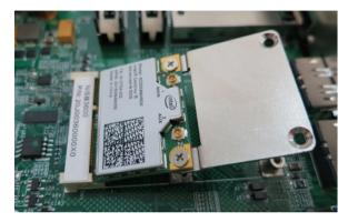
4. Push the module down and then secure it with mounting screws.
