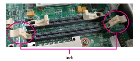
3. Insert the module into the socket at an 90 degree angle. Apply firm even pressure to each end of the module until it slips into the socket.
