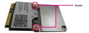
3. Insert the wireless LAN module into the Mini PCI Express slot at a 45 degree angle until the gold-plated connector on the edge of the module completely disappears inside the slot.
