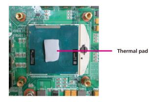
6. Fasten the CPU heatsink in its original place.
