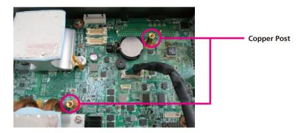
3. Secure the GPS bracket on the copper post.
