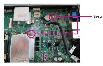
2. Fasten the copper post included in the accessory bag onto the screw holes.
