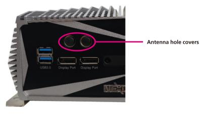
2. Insert the antenna jack through the antenna hole.
