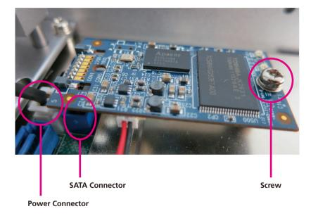
5. Fasten the screw on the top of copper post.
