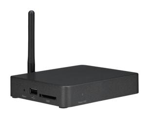
Powered by ARM<sup>®</sup> Cortex<sup>®</sup>-A17 quad core, NDiS B115 can play rich multimedia contents with low power consumption. NDiS B115 is enclosed in a compact chassis and can be easily integrated to display devices, such as LCD TV or PDP at site installation with HDMI display output (up to HDMI 2.0 support 4K2K 60Hz), Gigabit LAN. NDiS B115 is suitable as an entry level digital signage player for advertising, messaging, and brand promotion.
