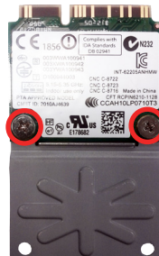
Join the WiFi module and the “mini half bracket” by using two screws.
