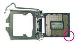
The CPU's notch will at the same time fit into the socket's alignment key.
