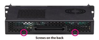
2. With the screws removed, lift up the cover and remove it from the chassis.
