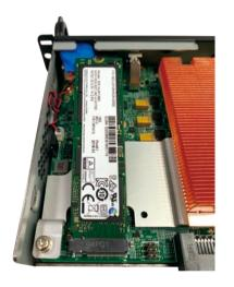
4. Push the module down and secure it with the screw removed in step 2.
