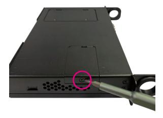
2. Remove the cover and locate the M.2 E key slot on the mainboard.
