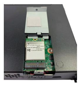
4. Push the module down and then secure it with a mounting screw.
