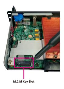
2. Remove the screw on the copper standoff. Put the screw in a safe place for later use.
