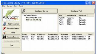
The user-friendly VxComm Driver/Utility allows users to easily turn the built-in COM ports of the PDS-5105D-MTCP series into standard COM ports on a PC. By virtue of its protocol independence, specialized OS and high flexibility, the PDS-5105D-MTCP series is able to meet the demands of any network-enabled application.
