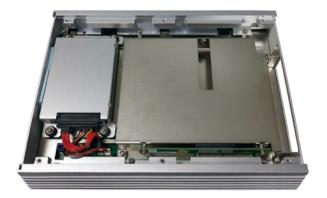
2. Unscrew the HDD bracket and lift it up.
