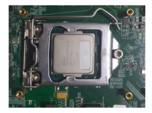
8. Take out the thermal pad from the accessory bag and remove the release paper on the thermal pad. Place the thermal pad on the CPU.
