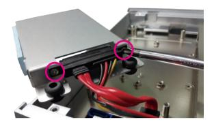
4. Place the HDD into the HDD bracket and secure the HDD with screws.
