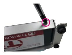
5. Connect the SATA connector to the HDD and secure the HDD bracket back to its original location.
