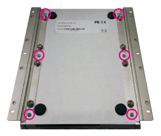
2. Remove the screws then lift up the bottom cover and remove it from the chassis.
