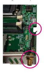
3. Unscrew the HDD bracket and lift it up.
