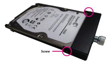
4. Put the HDD back into the slot gently, then tighten the screw to secure it.
