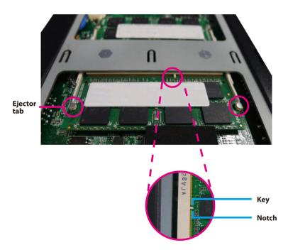
3. Insert the module into the socket at an approximately 30 degrees angle. Apply firm even pressure to each end of the module until it slips down into the socket. The contact fingers on the edge of the module will almost completely disappear inside the socket.
