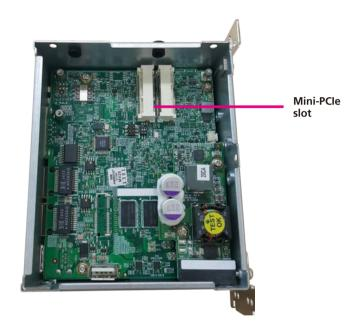
2. Insert the mSATA module into the mini-PCIe slot at 45 degree angle until the gold-plated connector on the edge of the module completely disappears into the slot.
