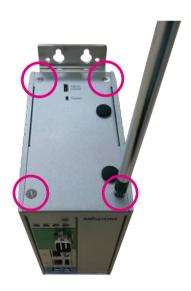
2. Remove the screws on the bottom chassis.
