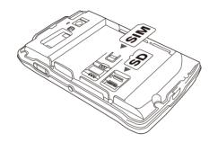
5. Push the metal cover backward and lift the metal cover. Then put the SD card into the socket, close the metal cover and push forward till click sound.
