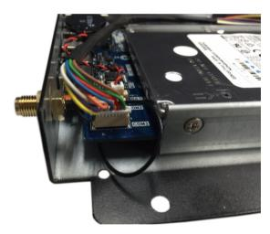
6. Insert the ring onto the antenna jack end of the cable.
