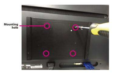
2. Secure the device to the wall mount bracket with screws.
