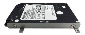
3. Place the SATA drive in the chassis and connect the SATA data connector, then use the provided mounting screws to secure the drive in the chassis.
