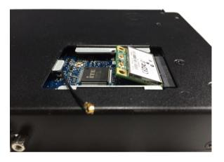
4. Secure the module with mounting screws and attach one end of the RF cables onto the module.
