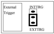
The A-822PGL/PGH supports two trigger type, **internal trigger** and **external trigger**. The external trigger comes from **ExtTrg**, **CN3** pin 17. There are two types of internal trigger, **software trigger** and **pacer trigger**. The details information is given in section 2.4.8.
