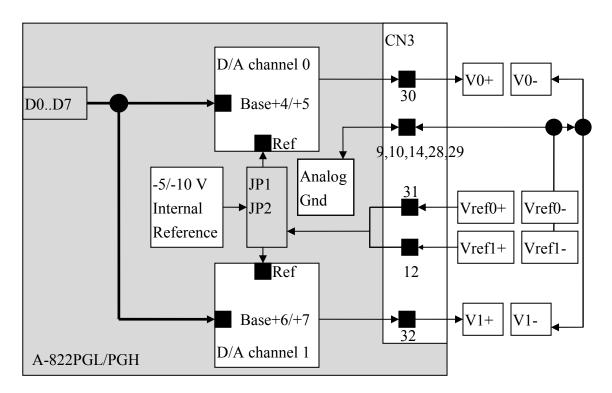
NOTE: The DA output latch registers are designed as "double buffer" structure. The user must send the low byte data first, and then send the high byte data to store the DA 12 bits digital data. If the user only sends the high byte data, then the low byte data will be still the previous value. Also if the user send high byte first then send low byte, the low byte data of DA are still hold in the previous one.
