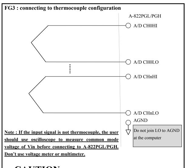
**CAUTION**: In Fig3, the maximum common mode voltage between the analog input source and the AGND is 70  $V_{p-p}$ , so the user must make sure that the input signal is under specification first. If the common mode voltage is over 70  $V_{p-p}$ , the input multiplexer will be damaged forever.
