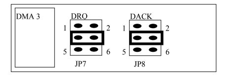
**The DMA channel can not shared.** The A-822 software driver can support 8 different boards in one PC based system, but only **two of these boards** can use DMA transfer function.
