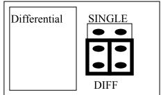
The A-822PGL/PGH offer 16 single-ended or 8 differential analog input signals. The JP3 select single-ended/differential. The user can not select single-ended and differential simultaneously.
