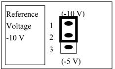
Select (-5 V) : D/A voltage output =  $0 \sim 5$  V (both channel)
