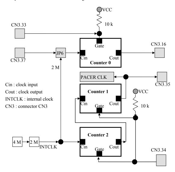
The counter0, counter1 and counter2 are all 16 bits counter. The counter 1 and counter 2 are cascaded as a 32 bits timer. This 32 bits timer is used as <u>pacer timer</u>. The software driver, A-822\_Delay(), use counter 0 to implement a machine independent timer for settling time delay (sec. 2.4.6 and sec. 2.4.7). If user doesn't use A-822\_Delay(), the counter0 can be used as a general purpose timer/counter.
