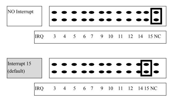
The interrupt channel <u>can not be shared.</u> The A-822 software driver can support 8 different boards in one system but only **2 of these cards** can use interrupt transfer function.
