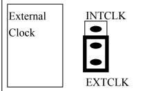
The A-822PGL/PGH has 3 independent 16 bits timer/counter. The cascaded counter1 and counter2 are used as **pacer timer**. The counter0 can be used as a user programmable timer/counter. The user programmable timer/counter can select **2 M internal clock** or **external clock ExtCLK, CN3 pin 37**. The block diagram is given in section 2.6. The clock source must be very **stable.** It is recommended to use internal 2 M clock.
