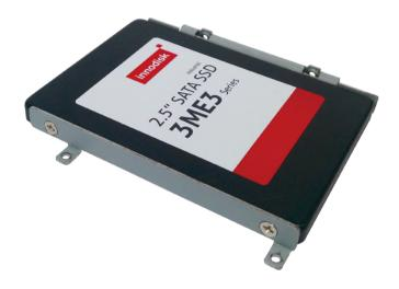
2. Place the SATA drive in the chassis and connect the SATA data connector, then use screws to secure the drive in the chassis.
