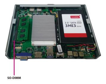
2. Push the module down until the clips on both sides of the socket lock into position. You will hear a distinctive "click" sound, indicating the module is correctly locked into position.
