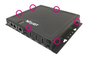
2. With the screws removed, lift up the cover and remove it from the chassis.
