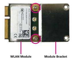
2. Insert the wireless LAN module into the mini-PCI Express slot at a 45-degree angle until the gold-plated connector on the edge of the module completely disappears inside the slot. Push the module down and then secure it with mounting screws.
