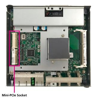
2. Insert the module into the mini-PCle slot at a 45-degree angle until the gold-plated connector on the edge of the module completely disappears into the slot.
