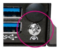
Specification of the round head screw: Round Head Screw Long Fei: p6#32T Nylok P6#32T Outer Teeth Washer Nylok
