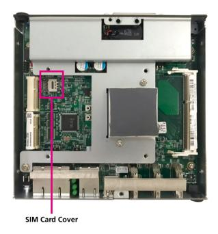
2. Release the cover and place the SIM card onto the holder.
