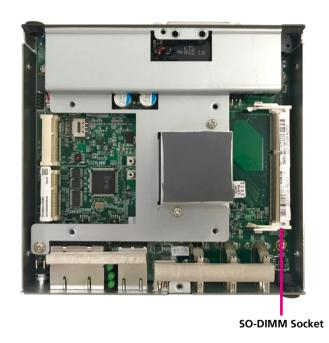
2. Insert the module into the socket at an approximately 30-degree angle. Push the module down until the clips on both sides of the socket lock into position. The ejector tabs at the ends of the socket will automatically snap into the locked position to hold the module in place.
