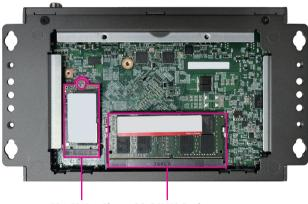
M.2 M Key Slot SO-DIMM Socket
