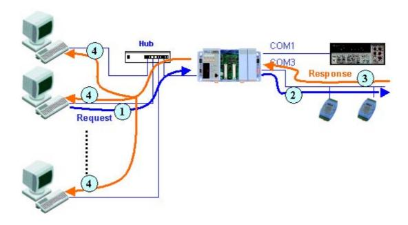
Condition 2: No clients send a request to Xserver to access devices. The Xserver echoes data from devices to every client which are connected to the 7188E/8000E.
