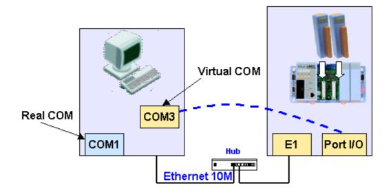
Step 3: Click the menu item "COM Port" to choose the COM port number, baudrate, and checksum. For example: COM3, 115200, 19200, 9600 and No-Checksum. (These settings depend on the 8000 series module's settings.)
