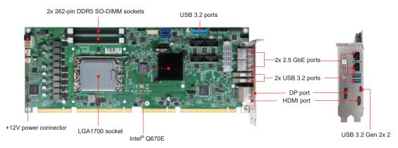
ROBO-8116G2AR-Q670E is based on Intel ® 600 series chipset and workstation
