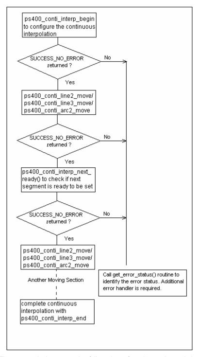
Figure 5 - typical programming follow-chart of continuous-interpolation
