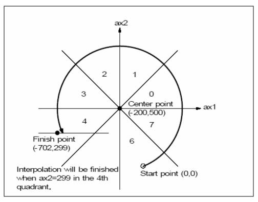
Figure 4 – finish-point checking of circular interpolation
